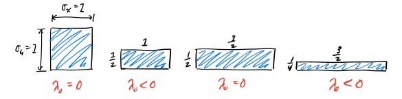
Figure 7.1.: From left to right: An undeformed element is already semi-definite. Squashing along y makes it indefinite. Stretching enough in x makes it semi-definite again. Squashing y even further pushes us back into indefiniteness.
