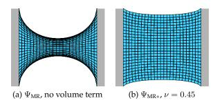
Figure 6.9.: Mooney-Rivlin, without a volume term (left), and with a volume term, but without rest stability (right). Same contraction problems as before: the mesh shrinks, even though no forces are being applied.
