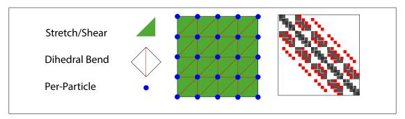
It makes sense to at least group the element forces by their mesh component domains, but we can go further. Instead of having a force element that handles each type of mesh feature, we aggregate overlapping forces onto the same fixed force element. Some elements naturally will be responsible for more force types than others and some will remain isolated.
