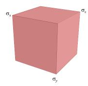
Figure 5.4.:  $III_{\mathbf{C}}^*$  is the squared *volume* of the cube:  $II_{\mathbf{C}}^* = (\sigma_x \sigma_y \sigma_z)^2$ .
