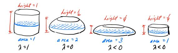
Figure 7.8.: From left to right: An undeformed volume is safely positive definite. As it is squashed by  $\frac{1}{2}$ , the cross-sectional area has to be at least 2 to prevent it from buckling. If this condition isn't met, the volume does not have base wide enough to hold up, and must buckle.
