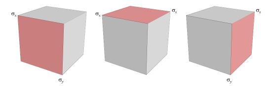
Figure 5.3.:  $II_{\mathbf{C}}^*$  sums up the squared *areas* of each side of the cube:  $II_{\mathbf{C}}^* = (\sigma_x \sigma_y)^2 + (\sigma_x \sigma_z)^2 + (\sigma_y \sigma_z)^2$ . I.e. it measures the overall face areas of the entire cube.
