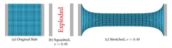
Figure 6.7.: Neo-Hookean material looks great under stretching (right), but produces a NaN and explodes under squashing.
