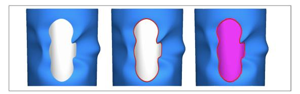
Figure 11.3.: An example the information GIA produces. Left to right: Two intersecting meshes. The intersection contour. The minimum colored area discovered by the flood fill.
