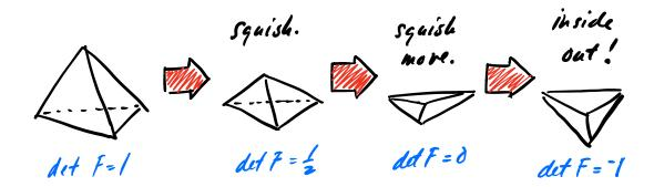
Figure 6.1.: A tetrahedron is sitting on a table (left). We squish its top vertex down (center, left) until it has been smashed into a pancake (center, right). We *keep pushing*, and the tetrahedron flips inside out! This is not physically possible, but it can *happen numerically*.
