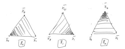
Figure D.2.: The basis functions are linear functions that are equal to one at their corresponding vertices and ramp linearly down to zero as the opposing edge is approached.
