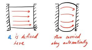
Figure 8.4.: The anisotropy direction a only needs to be defined at the rest shape. It gets automatically carried along as the object deforms.
