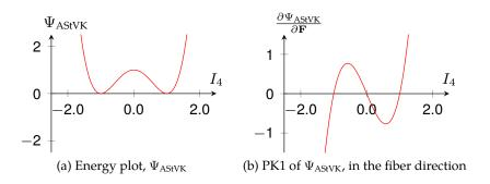
Figure 8.10.: Behavior of the  $\Psi_{AStVK}$  model, under stretching and compression.
