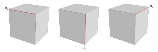
Figure 5.2.:  $I_{\mathbf{C}}$  sums up the squared lengths of each side of the cube:  $I_{\mathbf{C}} = \sigma_x^2 + \sigma_y^2 + \sigma_z^2$ . I.e. it measures the overall edge lengths of the entire cube.
