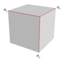
Figure 5.1.: The matrix  ${\bf F}$  describes the rotation and scaling of an infinitesimal cube of material. The singular values of  ${\bf F}$ , the  $\sigma_{\{x,y,z\}}$  labels above, describe the lengths of each side of that cube.
