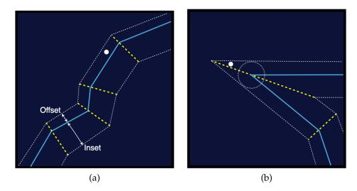
Figure 11.1.: Particle-Kinematic Face Cell Check: (a) Cell region containing a particle in the envelope. (b) Particle is inside the cell, but outside envelope.
